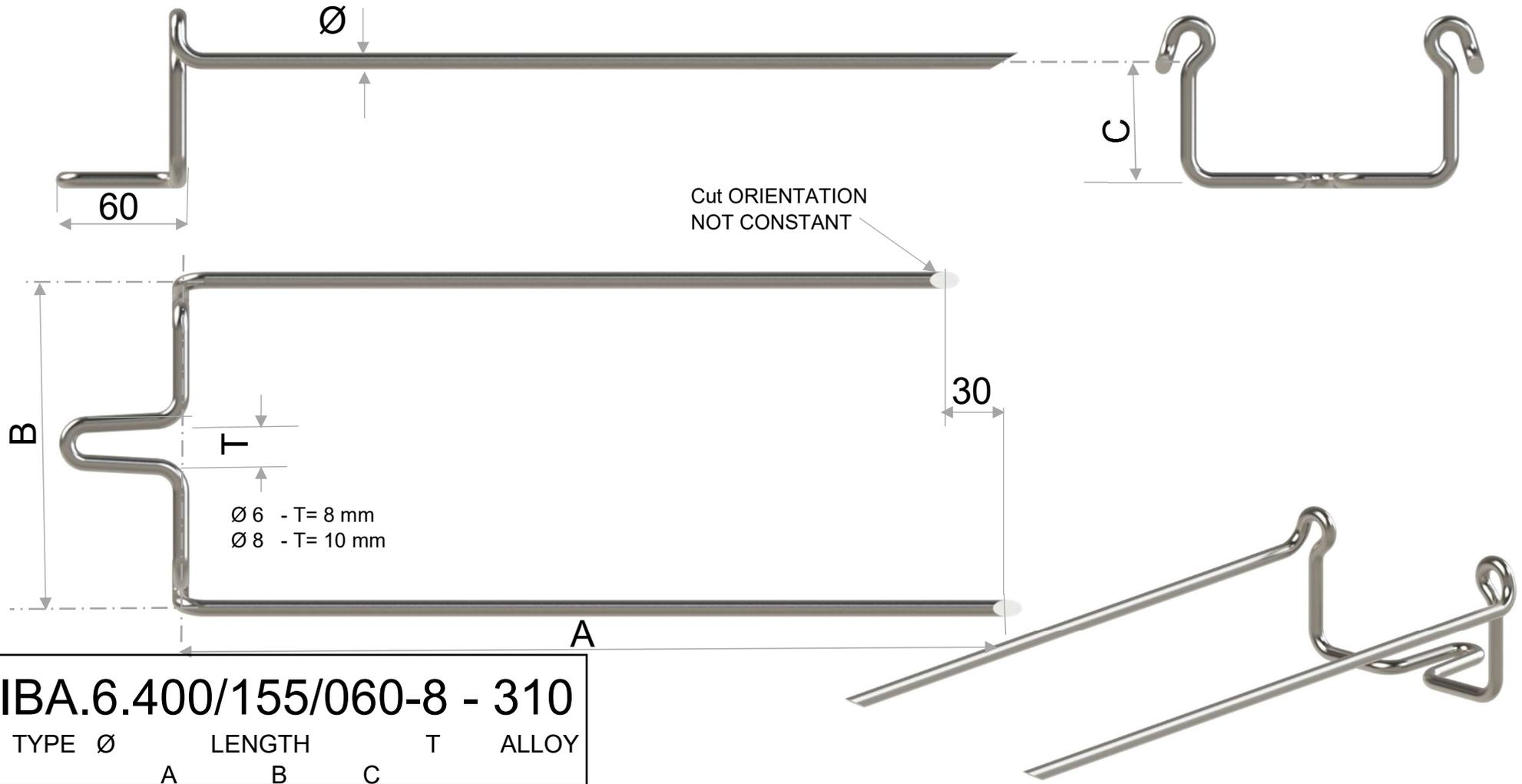
anchors are manufactured with a DIN EN 10278 (DIN 671) cold drawn wire, by robots using hydraulic tools. That allows minimizing bend marking and avoids micro cracks
